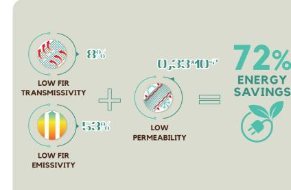
The permeability value of Noctis Thermo, determined by WUR, is 0.33\*10-7. This value is significantly lower than the permeability value of a traditional energy screen of approximately 0.6\*10<sup>-7</sup>. The combination of the low permeability, low FIR transmissivity and emissivity results in a screen that saves 72% energy. The interwoven yarn pattern ensures the necessary removal of excess moisture.
