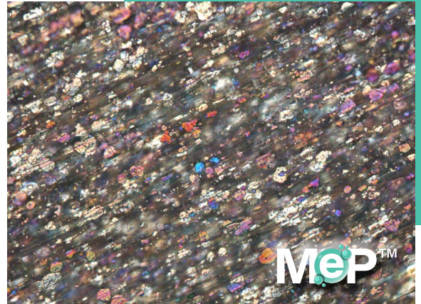
Microscopic photo of the aluminum particles encapsulated in PhormiTex Noctis Thermo
